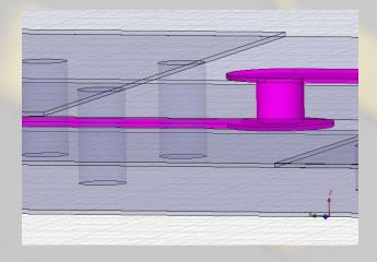
Taconic TSM-30 dielectric, each of two sections is 0.38mm in height
